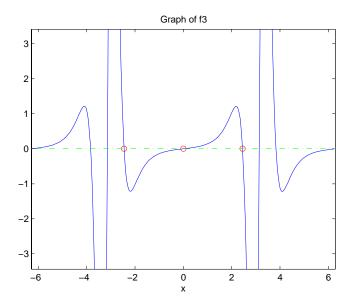
The red circles in the graph correspond to zerosd(1), zerosd(4), and zerosd(5). As you can see in the graph, there are also zeros at  $\pm \pi$ . The additional zeros occur because f'''(x) contains a factor of  $\sin(x)$ , which is zero at integer multiples of  $\pi$ . The function, solve(sin(x)), however, only finds the zero at x = 0.
